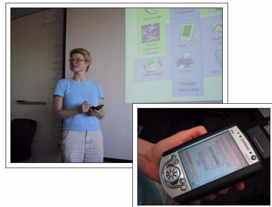
Figure 1 A user gives a presentation using Speakeasy. The network-enabled projector, and the filesystem on which the presentation resides, are Speakeasy components. The wireless PDA used to set up the connection automatically downloads presentation controls.
