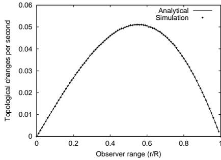
Figure 1: TCR for a static node at center of circular area and a RWP node moving at  $v = 5$  m/s.
