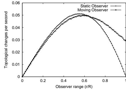
Figure 3: Comparison of TCR for static node at center and a moving RWP node.
